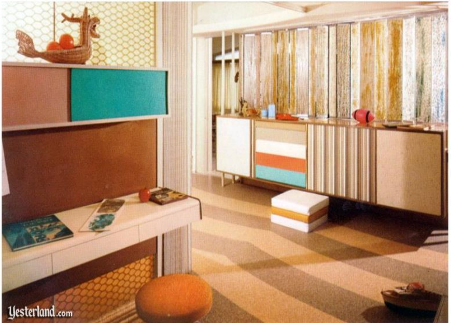
Partitions in children's room utilize folding plastic screen, laminated and molded plastic cabinets, honeycomb-reinforced plastic panels.
