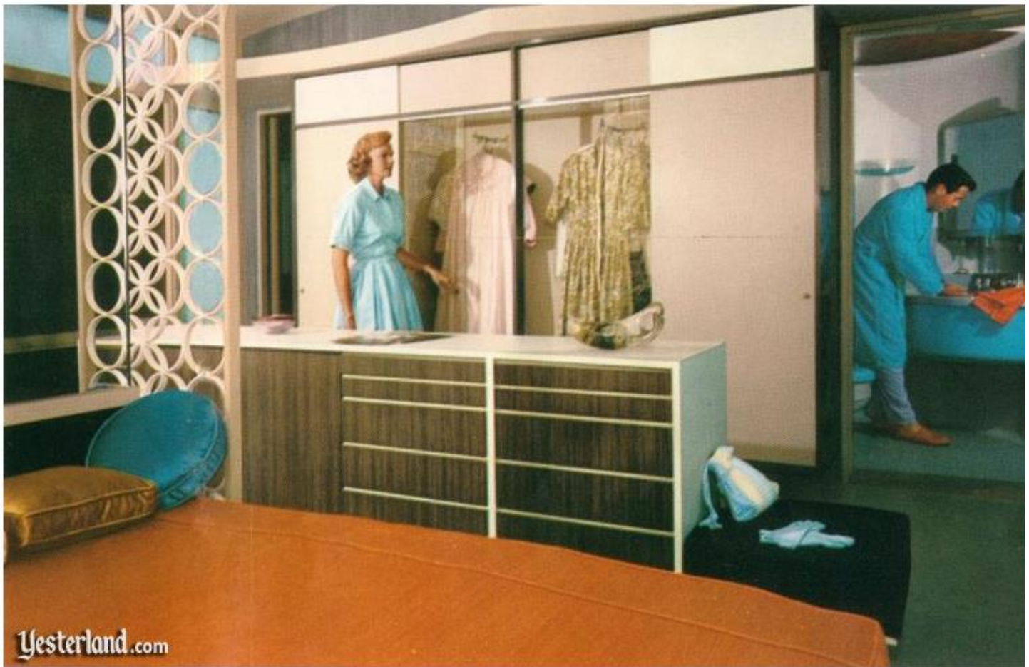
Decorative safety glass doors form front master bedroom storage units; one-piece molded plastic bathroom is at right. Plastic grillwork, cabinets form room divider.
